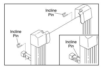
**CAUTION:** Before using the treadmill, make sure that both incline legs are at the same height. Do not use the treadmill with the incline pins removed. After you have adjusted the incline legs, lower the treadmill (see HOW TO LOWER THE TREADMILL FOR USE on page 11).
